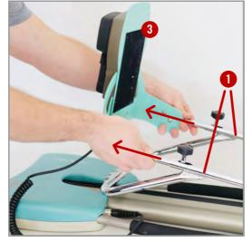
STEP 6 Rotate foot plate 3 and slide it parallel to bars for shipping.
